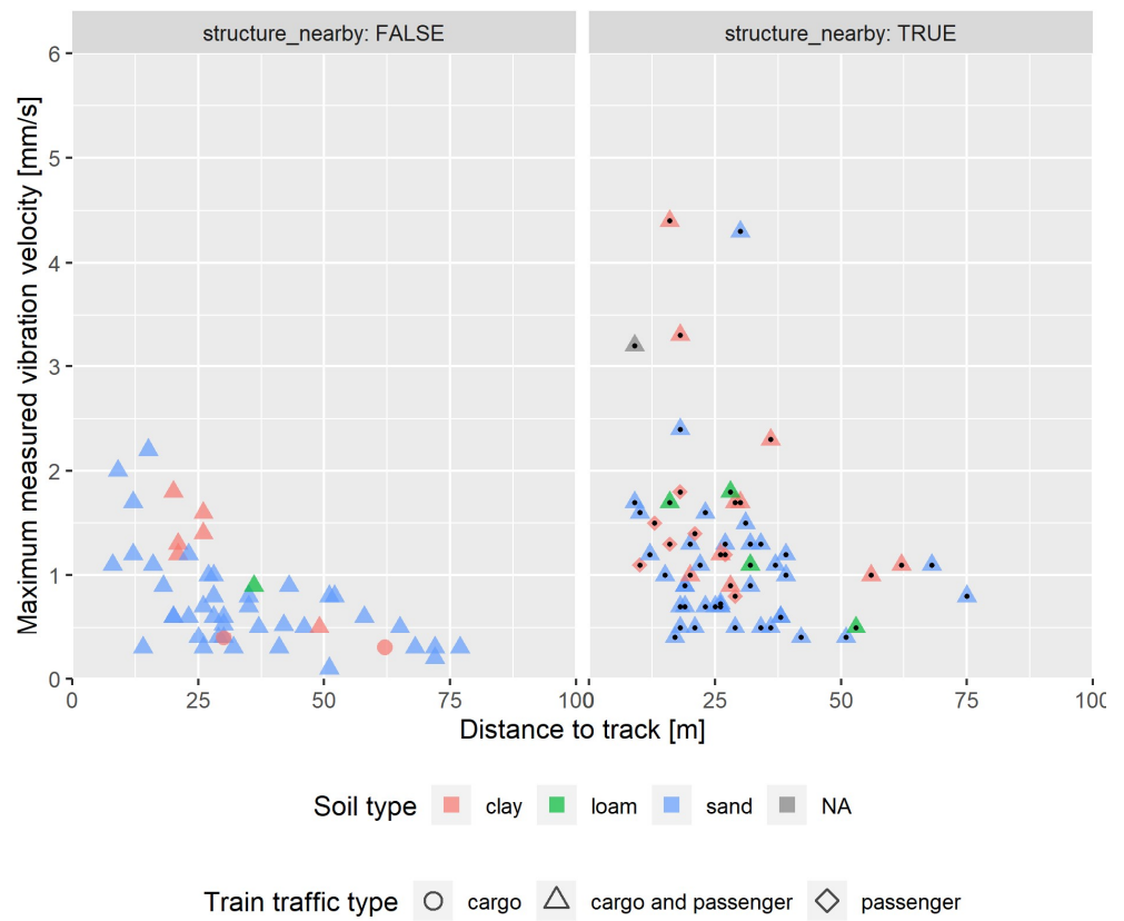
Figure 2-4: Visualization of the effect of soil type and train type on the attenuation of maximum vibration velocity over distance. The black dots inside the markers indicate if there is a structure nearby (Overweg of Kw = true), the absence of a dot indicates that there is no structure nearby. The two plots are combined in Figure 2-5. Data: N-M-SM.
