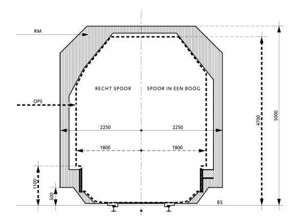
In case of doubt, One-Stop-Shop BV can calculate whether a statically measured load fits within the applicable reference gauges (adding margins as a result of the movement of loads and increase in curves).
