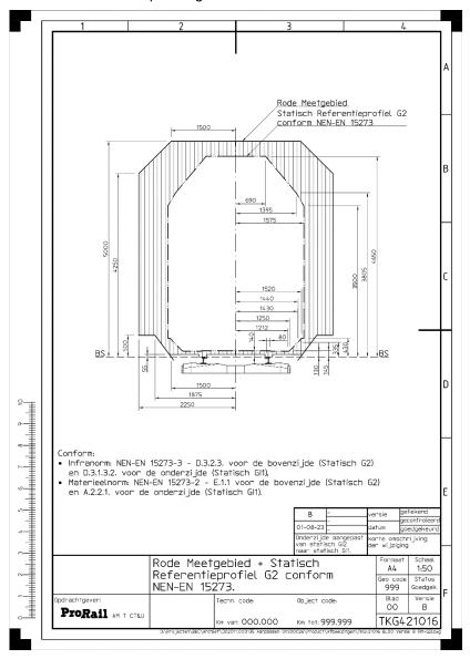
In case of doubt, the One-Stop-Shop for Exceptional Transport (OSS BV) can calculate whether a statically measured load fits within the applicable reference gauges (adding margins as a result of the movement of loads and increase in curves).
