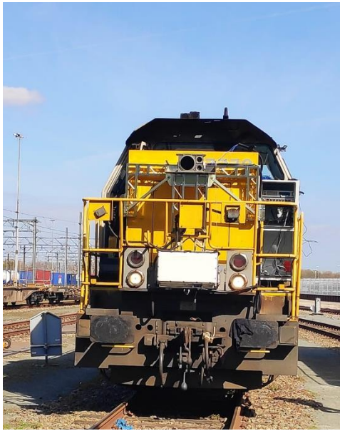
Figure 13 ODS on HDL77 (front view)
