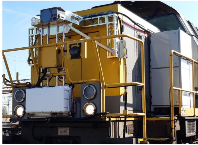
Figure 14 ODS on HDL77 (side view)
