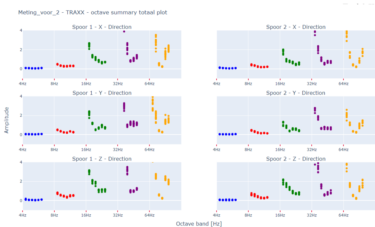
Figure 44 Vibration measurement data set 2 (Amplitude vs. octave bands) before track modification - TRAXX trains - Tracks 1 and 2, shown in the left and right figures, respectively.
