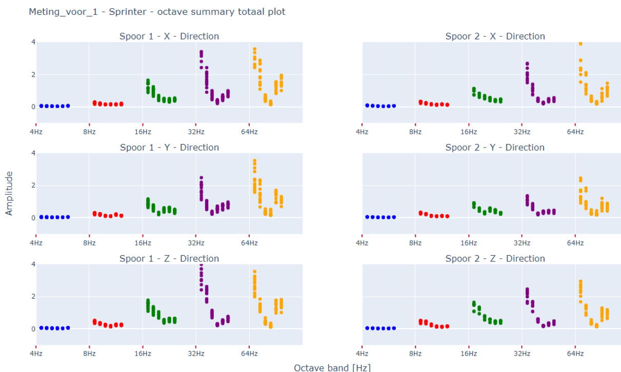
Figure 26 Vibration measurement data set 1 (Amplitude vs. octave bands) before track modification - Sprinter trains - Tracks 1 and 2, shown in the left and right figures, respectively.
