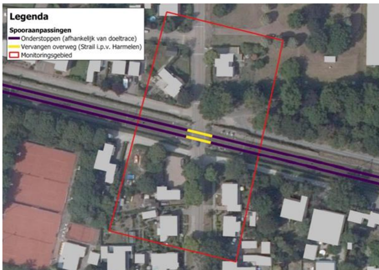
Figure 9 Geocode 123, between km. 6.295 en km. 6.370, concerning the level crossing replacement.
