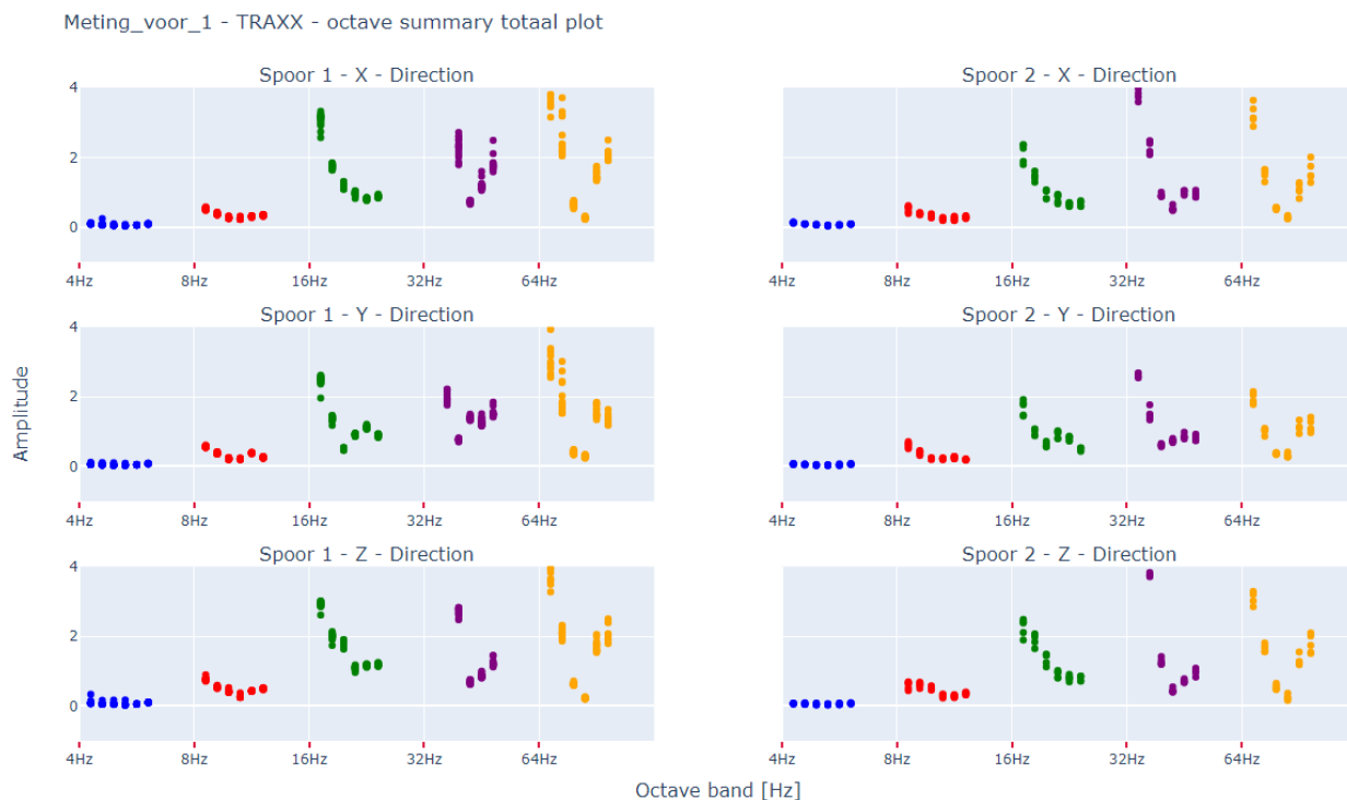
Figure 41 Vibration measurement data set 1 (Amplitude vs. octave bands) before track modification - TRAXX trains - Tracks 1 and 2, shown in the left and right figures, respectively.
