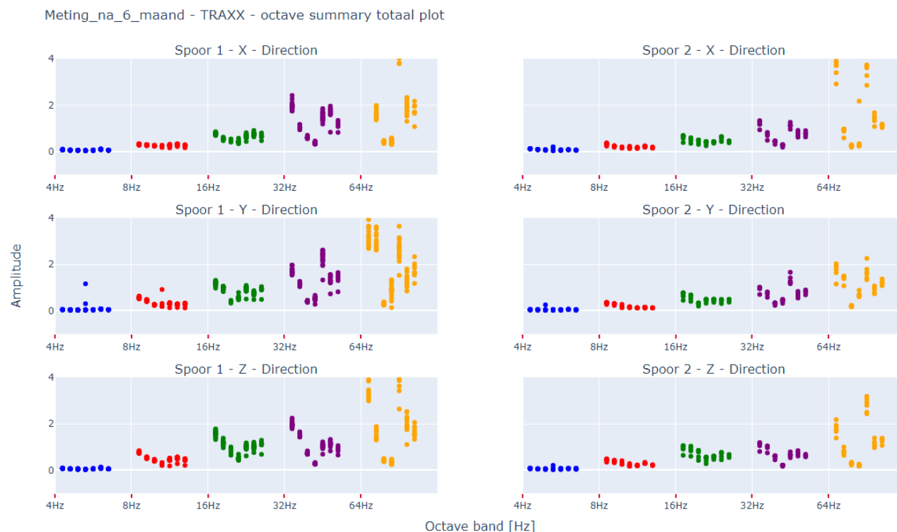
Figure 50 Vibration measurement data set (Amplitude vs. octave bands) 6 months after track modification - TRAXX trains - Tracks 1 and 2, shown in the left and right figures, respectively.
