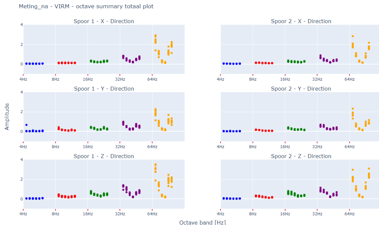
Figure 62 Vibration measurement data set (Amplitude vs. octave bands) directly after track modification - VIRM trains - Tracks 1 and 2, shown in the left and right figures, respectively.
