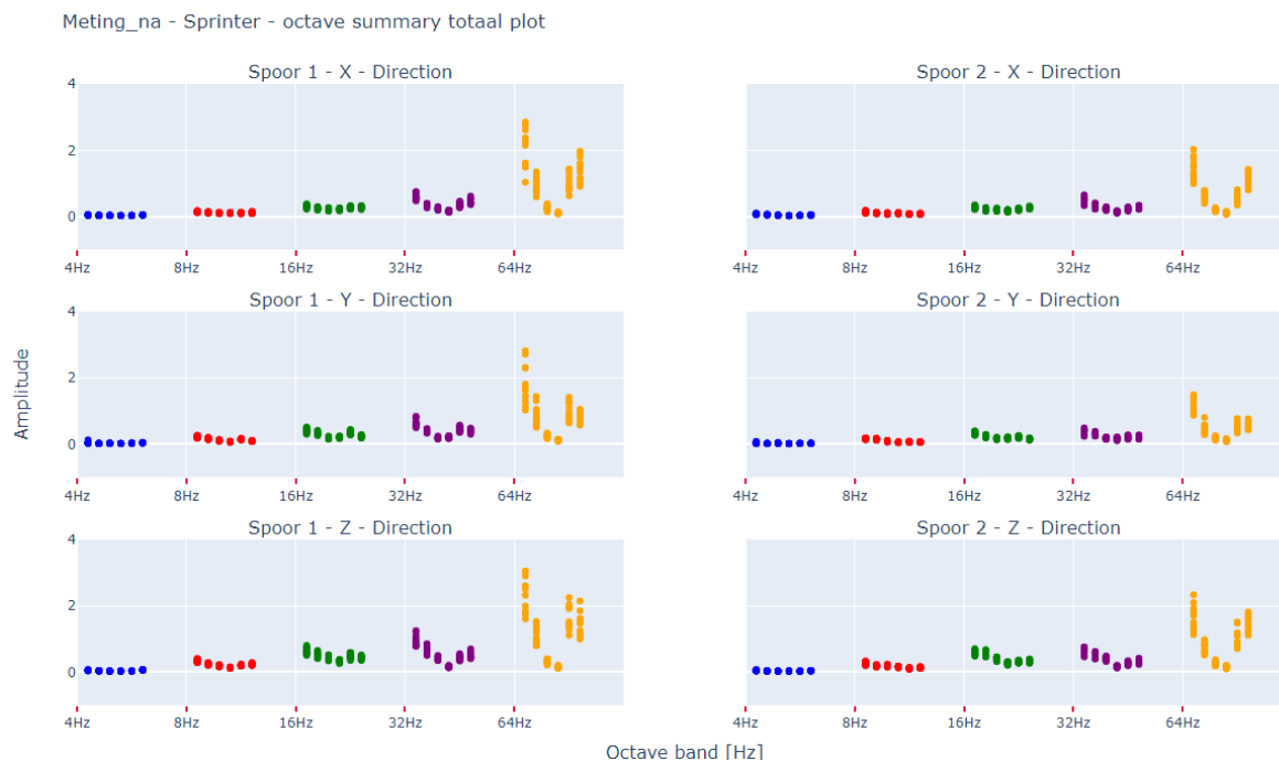
Figure 32 Vibration measurement data set (Amplitude vs. octave bands) directly after track modification - Sprinter trains - Tracks 1 and 2, shown in the left and right figures, respectively.
