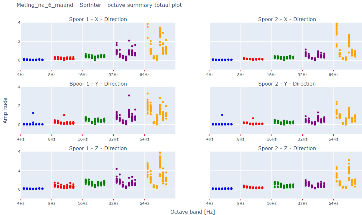
Figure 35 Vibration measurement data set (Amplitude vs. octave bands) 6 months after track modification - Sprinter trains - Tracks 1 and 2, shown in the left and right figures, respectively.
