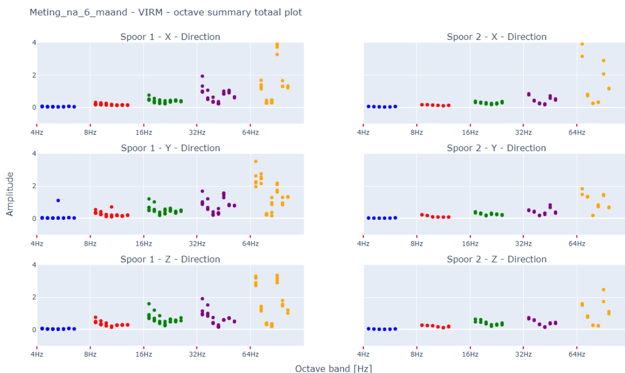
Figure 65 Vibration measurement data set (Amplitude vs. octave bands) 6 months after track modification - VIRM trains - Tracks 1 and 2, shown in the left and right figures, respectively.
