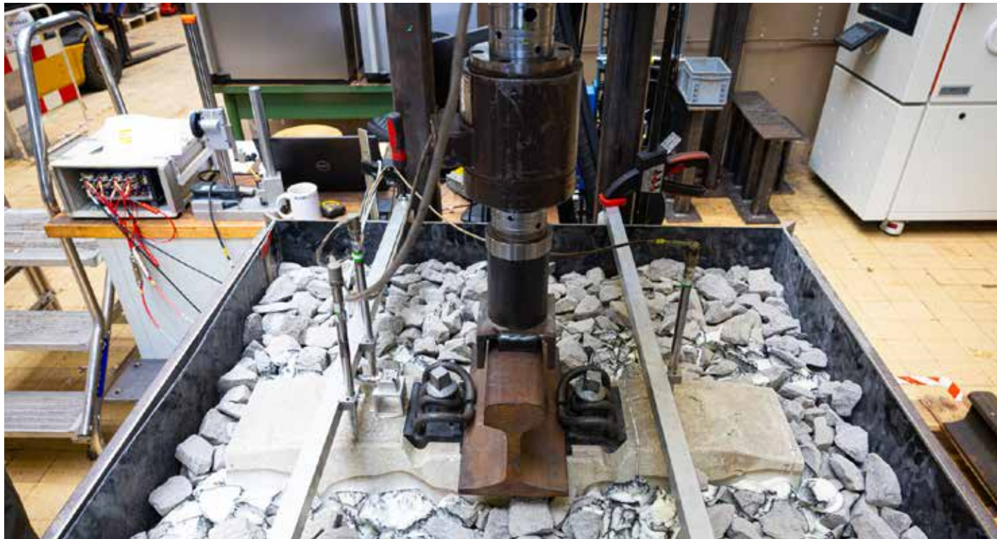
Figure 26 Test setup for foamed ballast
