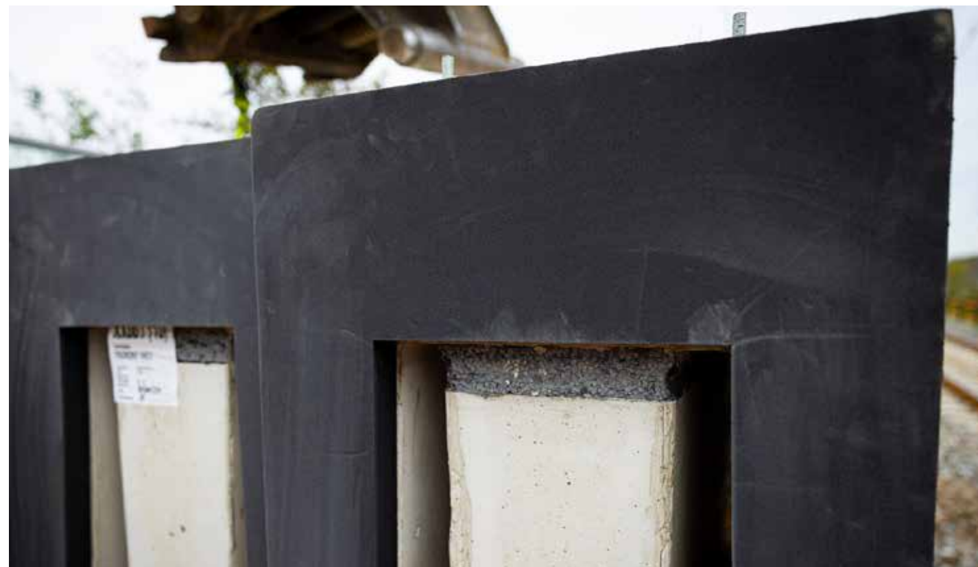
Figure 32 Cross-section of MetaBarrier showing internal mass-spring system
