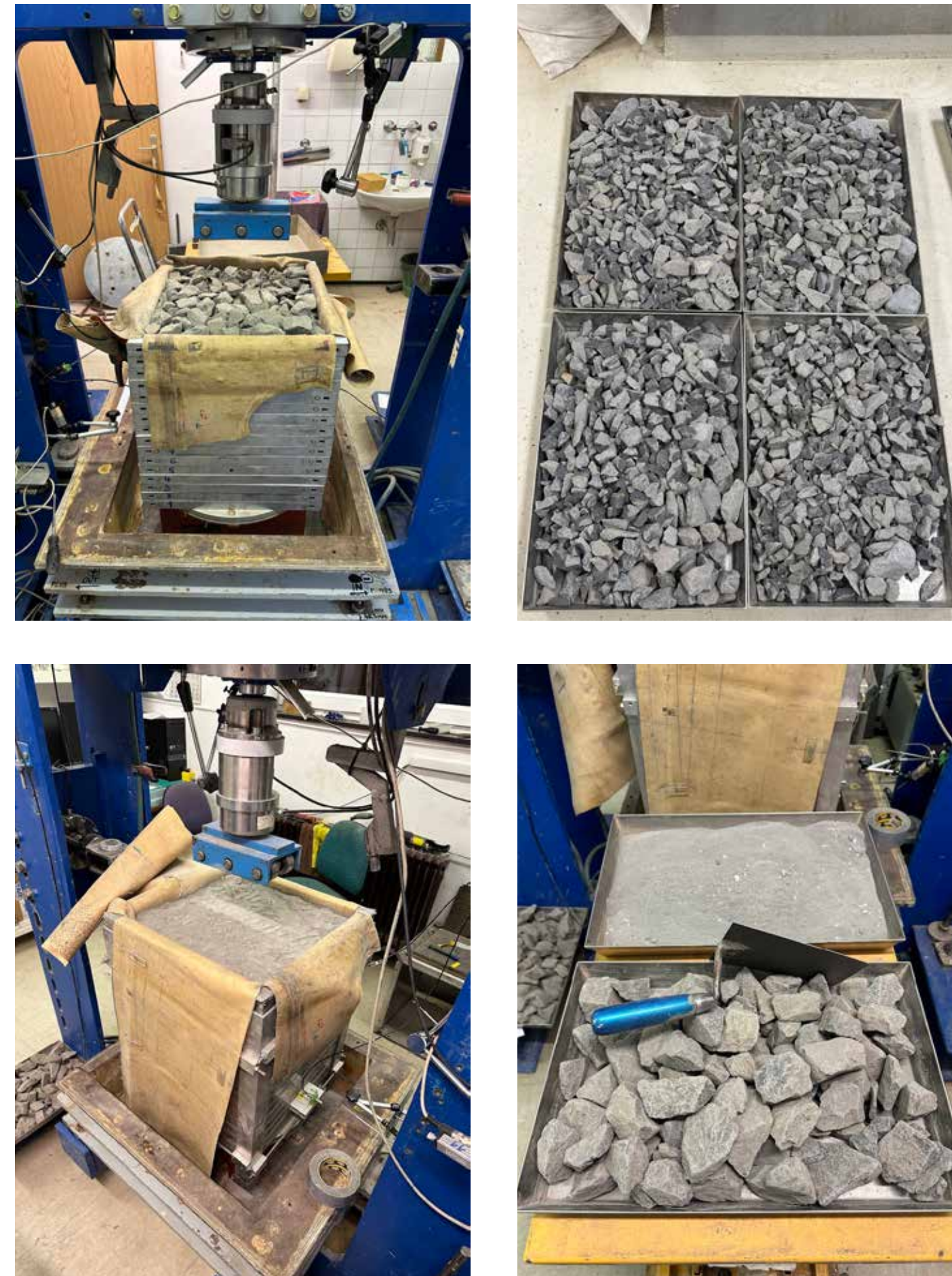
Figure 38 Test setup for mechanical ballast testing
