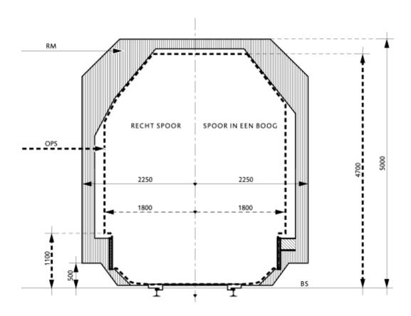
In case of doubt, One-Stop-Shop BV can calculate whether a statically measured load fits within the applicable reference gauges (adding margins as a result of the movement of loads and increase in curves).
