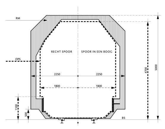
In case of doubt, the One-Stop-Shop for Exceptional Transport (OSS BV) can calculate whether a statically measured load fits within the applicable reference gauges (adding margins as a result of the movement of loads and increase in curves).
